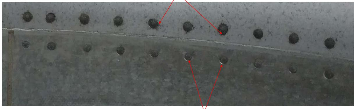
Corrosion of the inner Barrel is causing the barrel to Bulkhead attachment Hi-Lok pins to start pulling through into the surface due to the material expanding as the corrosion build up.
